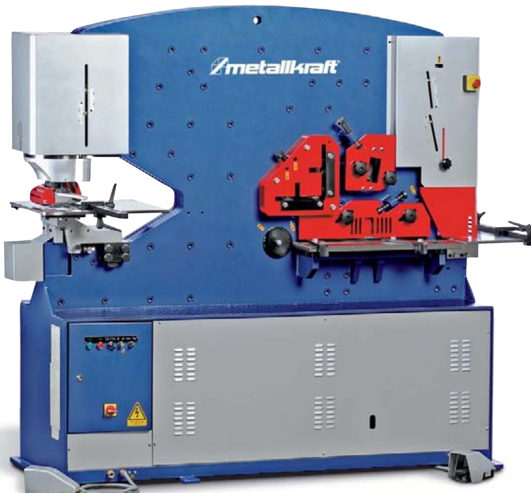
HPS 55/80/110 two cylinder type for independent working with two foot pedals
