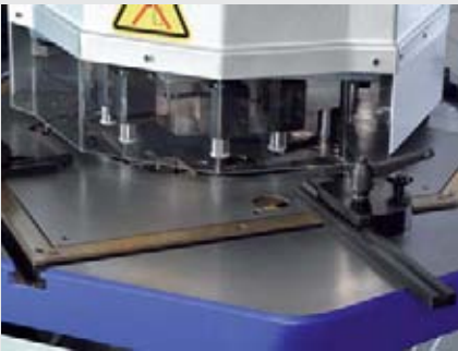
Working table with T-slots and immersed scales
