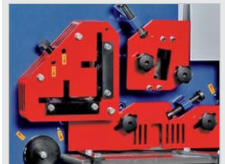
Angular steel station · angle of 45/90° · with 1000 mm rear stop · for HPS 45 manually all others with automatic cutting release
